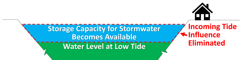
Figure 4. Storage capacity for stormwater (shown in blue) is available when the incoming tide is blocked. When the tide gate closed at low tide, the incoming tide is blocked and therefore storage capacity in Lake Windsor is available for stormwater flows.
