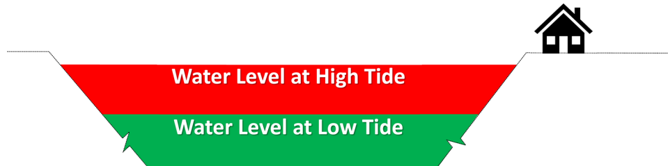
Figure 2. At high tide (shown in red), the storage capacity in Lake Windsor is dramatically reduced.
